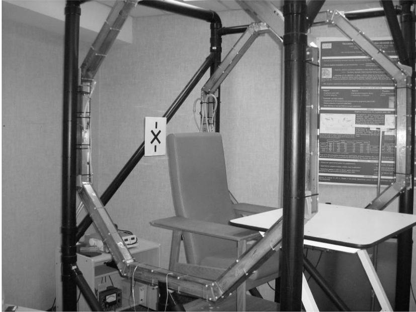
Figure 1 – The MF exposure apparatus.
